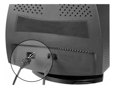
5 Plug the other end of the power cord into a correctly grounded electrical outlet.O
